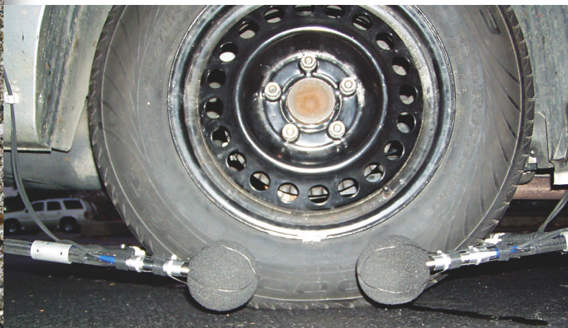
This on-board-sound-intensity-measurement system takes readings in the airflow (parallel with the vehicle) at the front and rear of the tire's contact patch.
