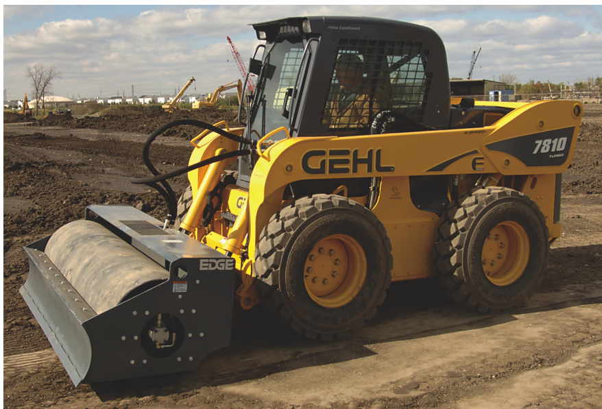
The 84-inch EDGE vibratory roller proved a serious attachment for the 7810E.
