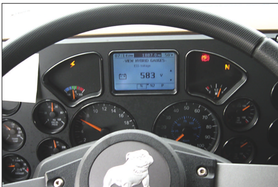
The voltmeter showed charge state of ultracapacitors; voltage varied between 580 and 610, with an aimed-for average of 600.
