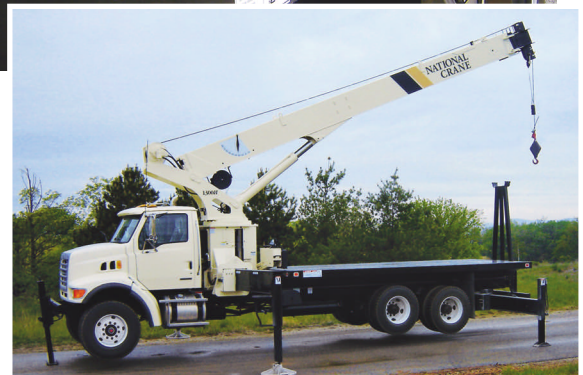
Above: Easy Reach control console folds in-line with the crane turret for transport. Operators can then easily access the truck bed.
