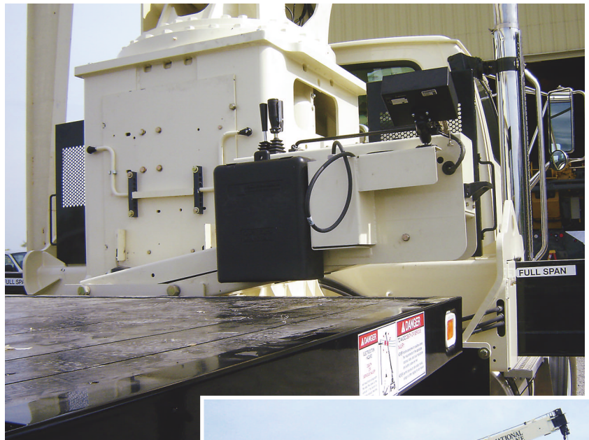
Above: Easy Reach control console folds in-line with the crane turret for transport. Operators can then easily access the truck bed.
