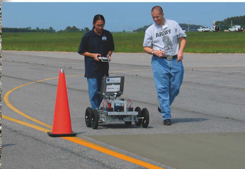
RoboTex, a robotic texture-measuring system developed by The Transtec Group, projects a laser line approximately 4 inches wide, thus generating a detailed, three-dimensional texture map. Photo: The Transtec Group
