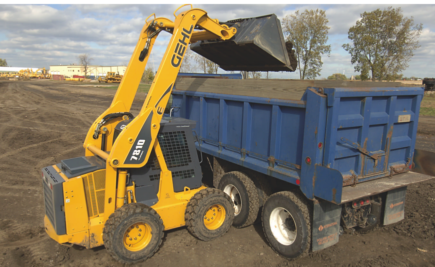
The 7810E had no problem getting up and over the 9-foot sideboards of this tandem-axle dump. Operator Tom Rush was impressed with both the machine's lift height and its digging ability.
